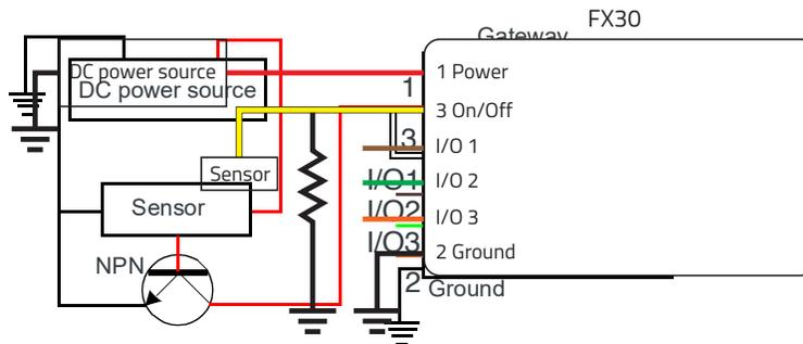
Figure 2-17: On/Off Installation (with sensor)
