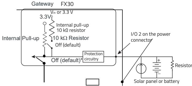
Figure 2-22: Analog Input Protection
