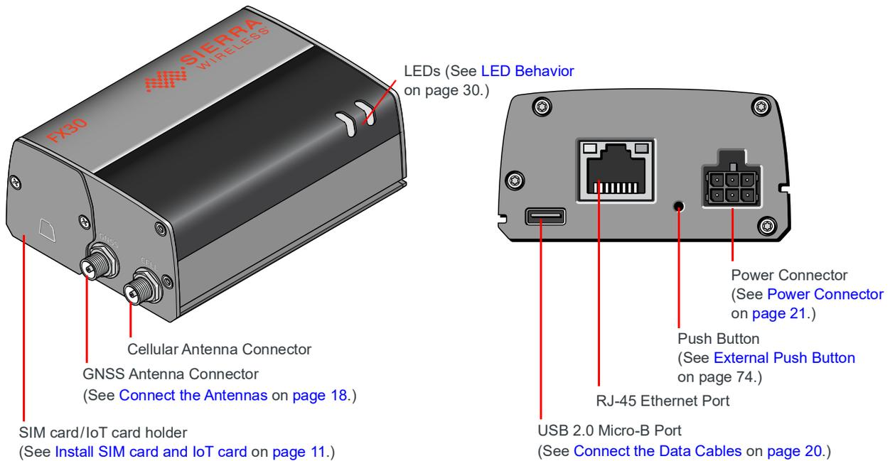
Figure 1-1: FX30 Connectors, LEDs and SIM Card Holder
