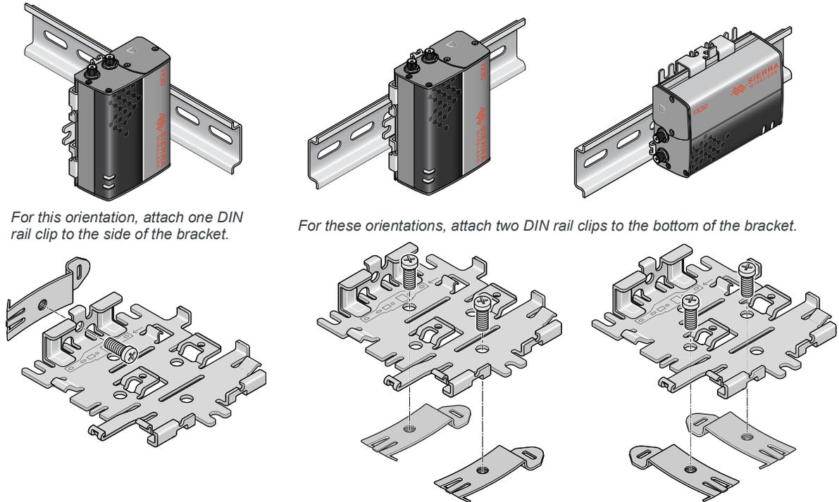
For this orientation, attach one DIN rail clip to the side of the bracket.
