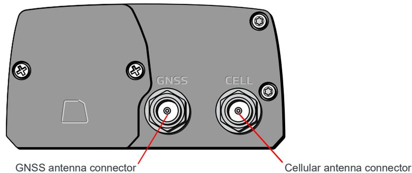
Figure 2-12: Antenna Connectors
