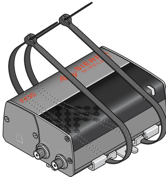
Figure 2-6: Inserting the ends of the ties
