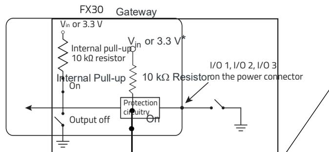
Figure 2-20: High Side Pull-up / Dry Contact Switch Input
